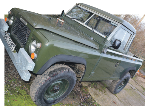
This 100-inch chassis prototype Land Rover from 1978 was built for the Swiss and French armies to test with a V8 engine and 24v electrics.
