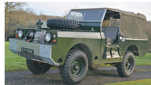
The amazing OTAL could cross rivers propelled and steered by its own wheels. Featuring an all-aluminium body and straight-six engine, it's an impressive and totally unique vehicle.
