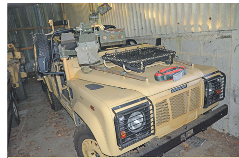
The Defender Wolf 110 WMIK (Weapons Mounted Installation Kit) demonstrator from 2002 enjoyed a 2.5-litre TDI engine, plus front- and top-mounted machine guns.
